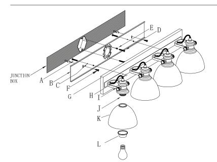
\*This fixture may be mounted on a wall or ceiling.
